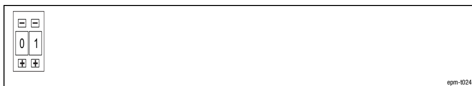
Abb. 5.2-3 Kodierschalter am CAN Gateway
